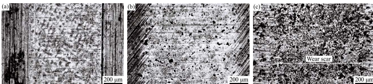
Figure 11. OM micrographs of pin wear scars for (a) SL 26, (b) A and (c) B samples
