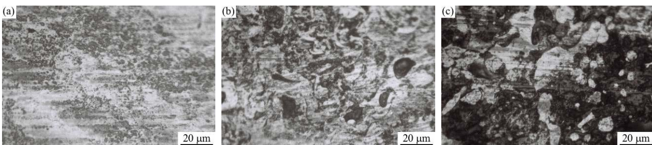
Figure 12. OM micrographs, at higher magnification, of pin worn surfaces for (a) SL 26, (b) A and (c) B samples
