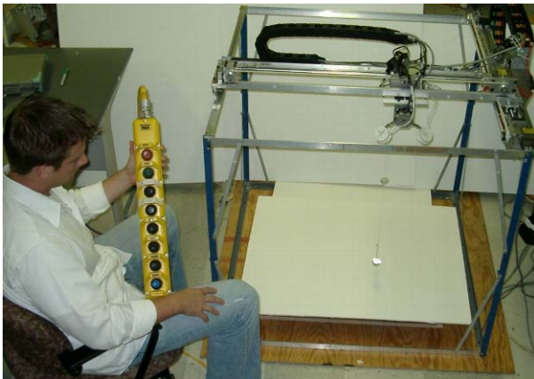
Figure 6. Portable bridge crane
