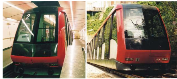
Figure 12. Montjuic reversible funicular in Barcelona, Spain [6]
