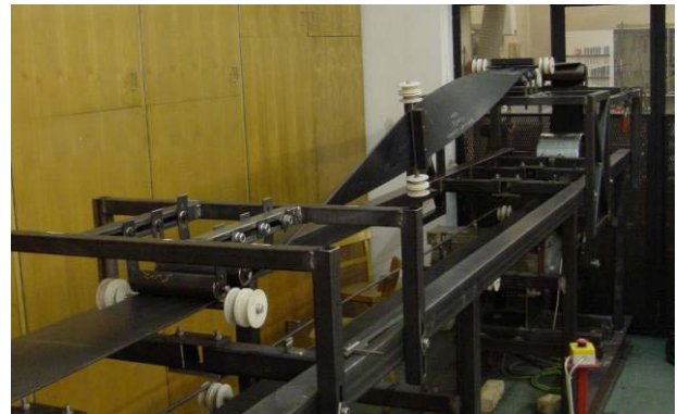
Figure 15. Test facility for the unguided belt turn-over
