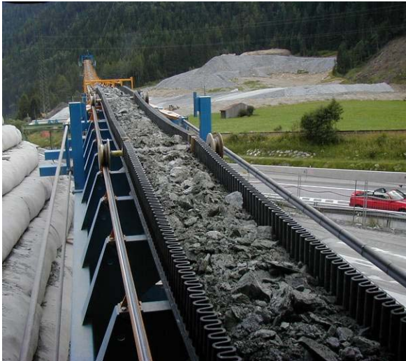
Figure 11. Detail view with track rope support frames and wheels rollers
