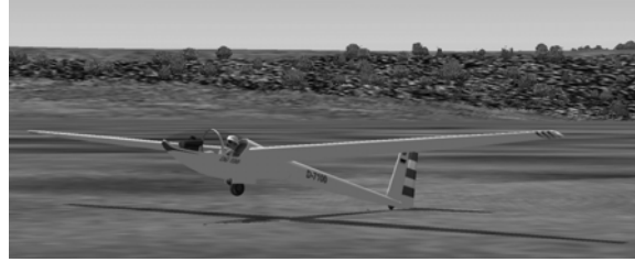
Figure 3. The DG-100 sailplane tail-first touchdown at V_{\text{stall}} (flight simulation for the visual presentation of the problem performed using the MS-FS9)
