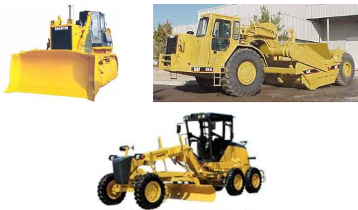
Figure 2. Constructive schemes of digging-transportation machines (bulldozer, scraper, grader)
