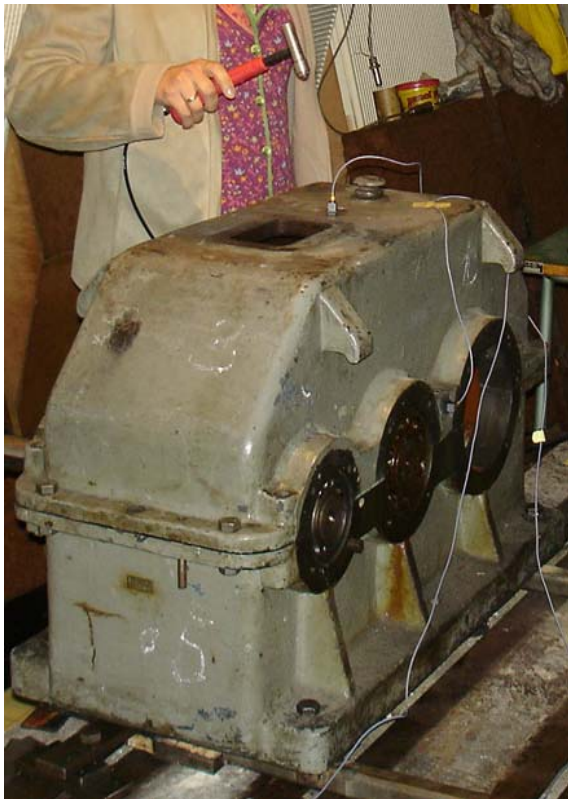
Figure 3. Gearbox housing modal testing
