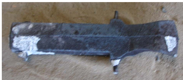
Figure 3. Casting of excavators tooth, immediately after shakeout from the mould
