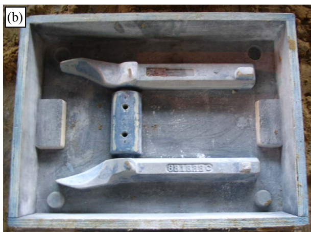
Figure 1. Patterns for moulds making: (a) shovel for asphalt mixer and (b) excavator tooth SRS 1700
