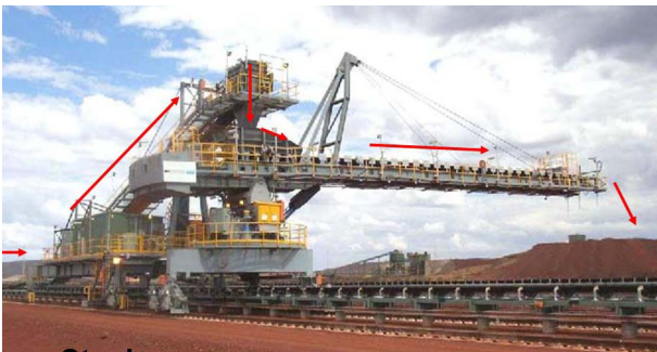
Figure 5. Transfer chutes for varying vertical and horizontal angles of discharge belt
