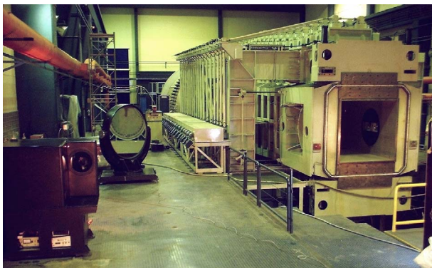
Figure 4. Diagonal mirror and optical receiver in Schlieren system configuration of the T-38 wind tunnel
