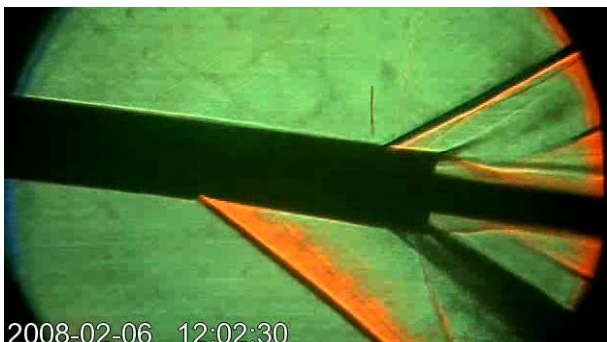
Figure 5. Flow visualisation around rear part of AGARD-B calibration model done using Schlieren method
