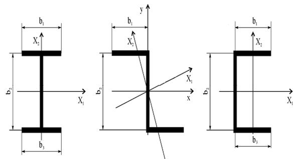
Figure 1. a) I-section; b) Z-section; c) Channel-section
