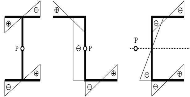
Figure 2. Sectorial coordinates for the I, Z and Channel cross-section
