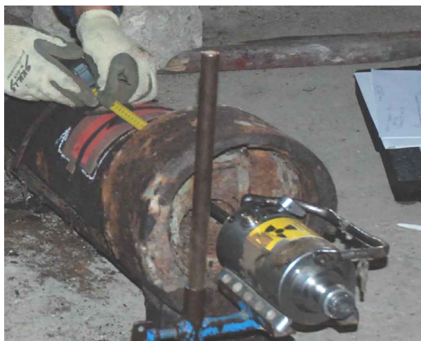
Figure 2. The cannon barrel preparation before the radiographic recording.
