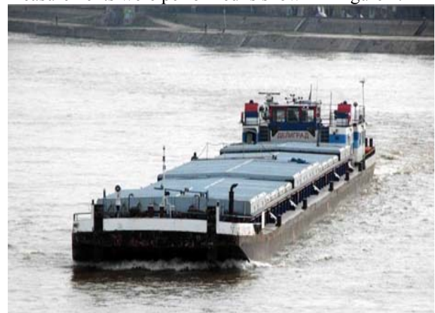
Figure 1. "Deligrad", owned by JRB (L=95m, B=11m, T=2.7m, Δ=2490t)
