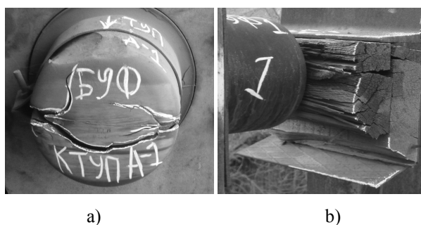
Figure 1. Damageability of bridge cranes rubber buffers and the ES: a – 16-ton bridge crane rubber buffer; b – the ES
