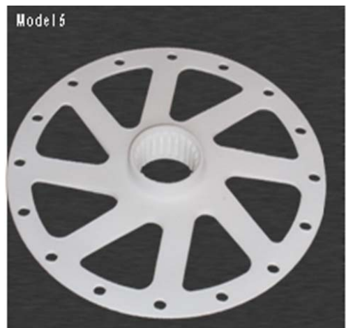
Figure 6. The suggested models of the rigid drive disc manufactured from polyamide material
