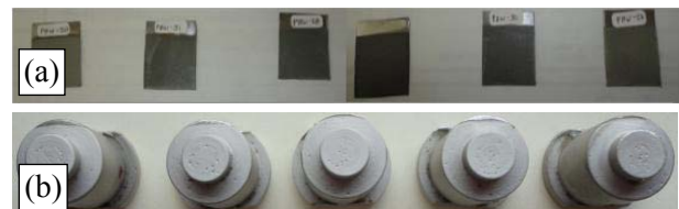
Figure 3. Specimens coated for: (a) corrosion tests and (b) tribology tests
