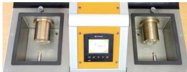
Figure 12. Two separate water tanks, nozzles and bearing housings
