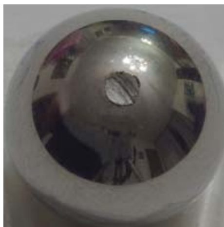
Figure 5. Photo of ball loaded with 120 kg after 60 minutes of wear test with a sample R3
