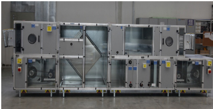
Figure 2. AHU for optimal energy efficient regimes testing – made by Soko Inženjering Belgrade
