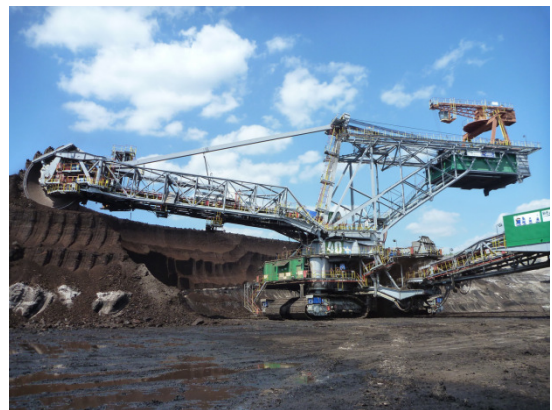
Figure 7 . Bucket wheel excavator SRs 2000
