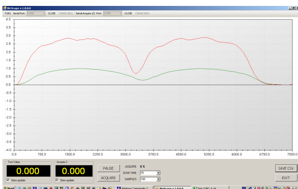
Fig. 8: Torque (upper curve) and current (lower curve) as functions of time under dynamic conditions.
