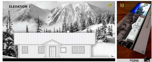
Figure 6. MH Petra: a) Elevation (marker); b) Augmented Reality presentation of elevation as 3D model
