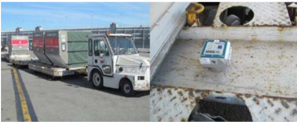
Figure 14. Instrumentation of dollies with data loggers [42].
