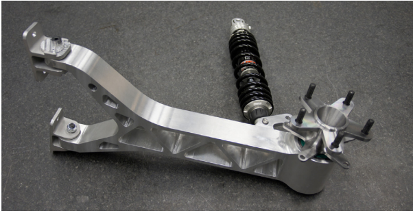
Figure 2. Rear trailing arm suspension by Solar Team Eindhoven [6]
