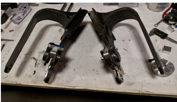
Figure 8. Adventure vehicle's wheel support in carbon fiber
