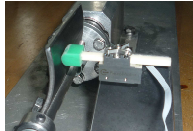
Figure 27. Linear motor mounted on the hybrid actuator
