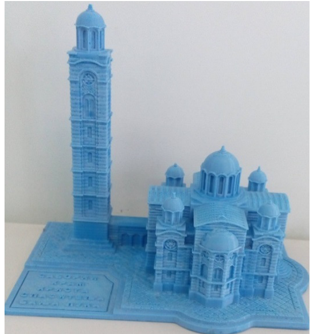
Figure 6. The religious object produced on the professional grade 3D printer Dimension Elite
