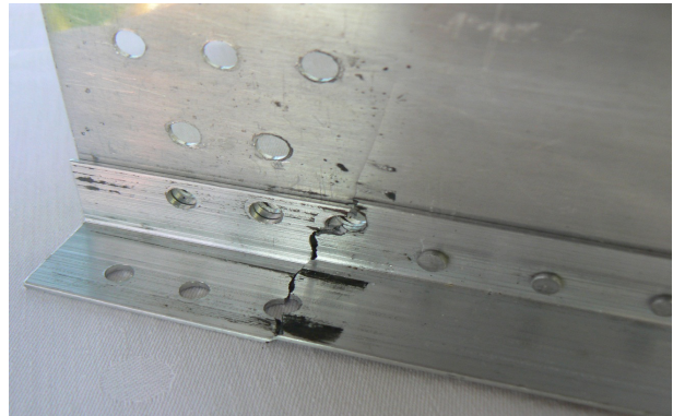
Figure 14. The crack at the left lower spar cap zone
