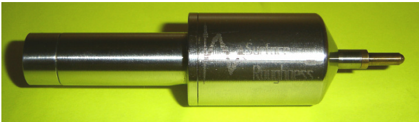
Fig. 3. A production version of AE profilometer in the form of a measuring probe head for the numerical control machines
