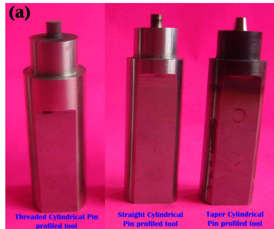
Figure 3. Photographic (a) front view and (b) tilted top view of the three distinct pin profiles of M35 HSS grade tools
