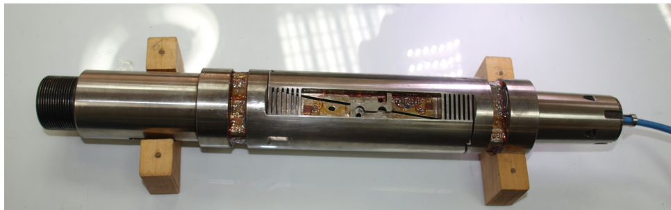
Figure 4. A 51 mm, 9 kN monolithic internal wind tunnel balance produced in VTI.
