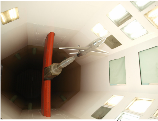
Figure 13. ONERA M4 calibration model (102 mm dia.) in the T-35 wind tunnel.
