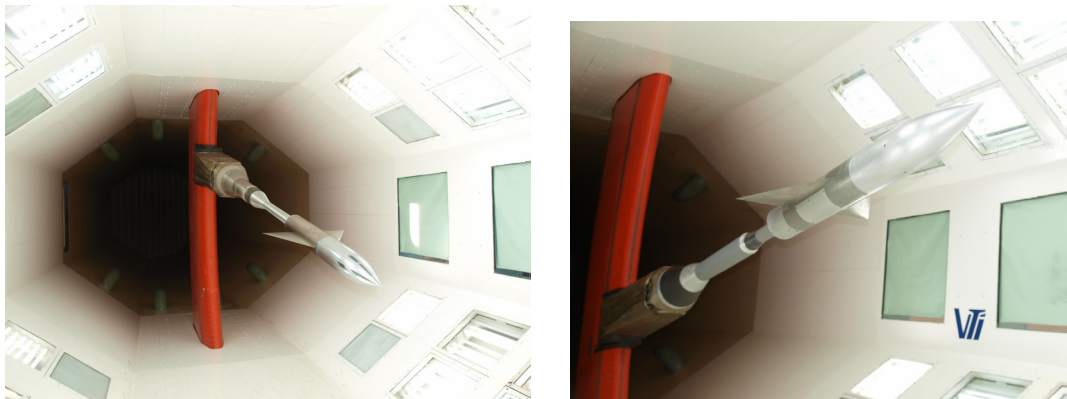
Figure 11. Two AGARD-B models (115.8 and 178 mm dia.) in the T-35 wind-tunnel.
