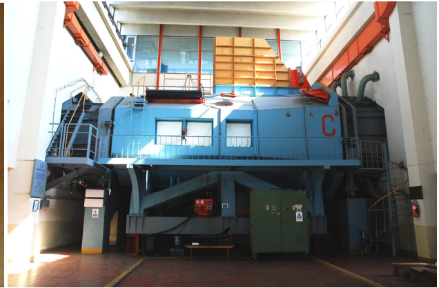
Figure 2. Variable-pitch-blades fan and tail-sting-support test-section of the T-35 wind-tunnel.
