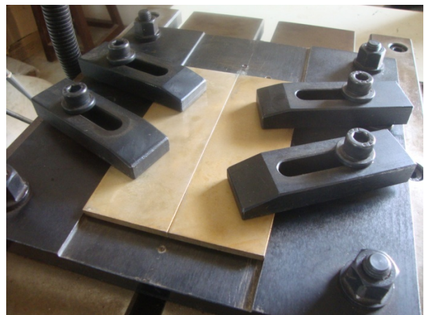
Figure 1. Photograph of the wrought AZ80A Mg alloy flat plates being firmly held in their respective position in the specially designed fixture of the FSW machine
