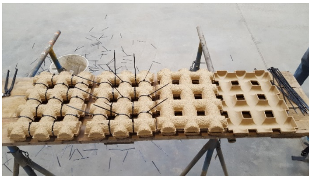
Figure 2. From right to left you can see the steps from the half shell to the interconnected void. We did a lot of handwork to seal them with laces. Photo by Jürgen Ries.
