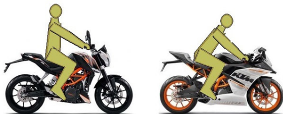
Figure 3. The rider's position in a street style motorcycle (on the left) and in a sport style motorcycle (on the right).
