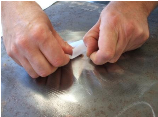
Figure 12: On the right: lower the tape again and compress the strain gauge on the sheet with a finger.
