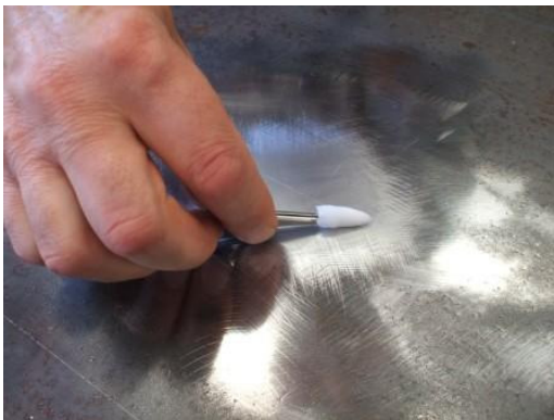
Figure 7: Degrease the area with a swab dipped in alcohol.
