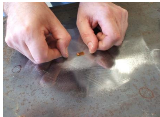
Figure 10: Overturn the adhesive tape, being careful to position it correctly on the sheet.
