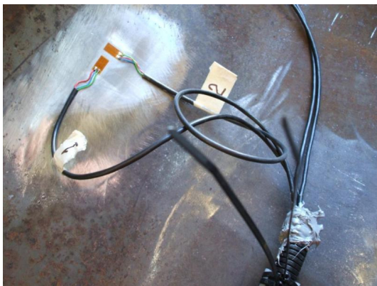
Figure 23: Place more than one strain gauge in the same area to ascertain the stress state.
