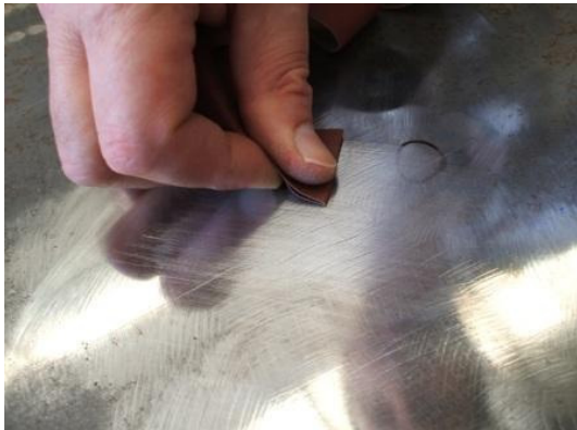
Figure 5: Sand the surface with grit sandpaper.
