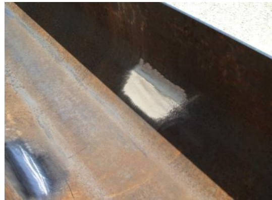
Figure 2. Prevent the abrasive disc from leaving furrows or depressions.
