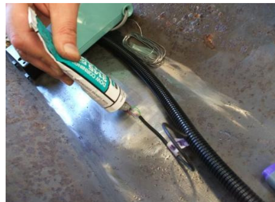
Figure 21: Apply a layer of silicone to protect the strain gauge.
