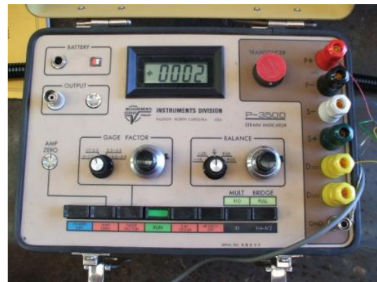
Figure 20: Connect the cables to the control unit and acquire the balancing values.
