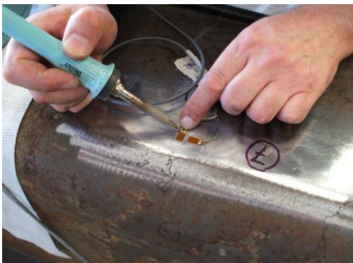
Figure 18: Solder the signal cables to the strainers of the strain gauge.
