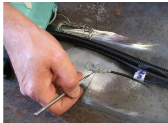
Figure 22: Squeeze the edges of the silicone firmly to isolate the contact area.
