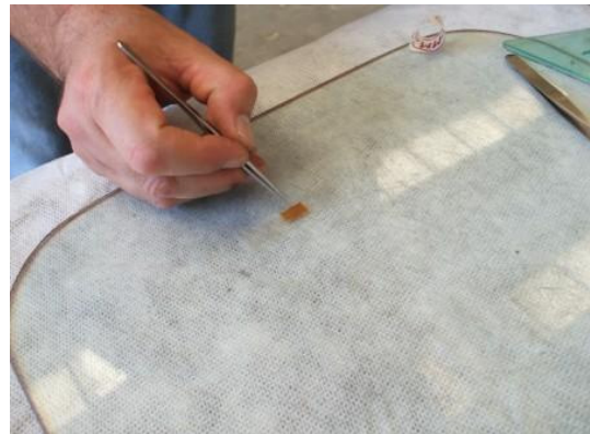
Figure 9: Remove the strain gauge from the package and place it upside down on a strip of adhesive tape.
