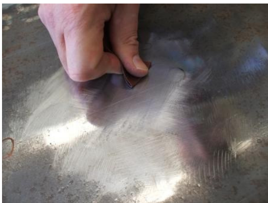
Figure 6: By making passes with orthogonal directions, super smooth surfaces are obtained.
