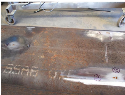
Figure 27: Provide strain gages placed in stand-by that intervene in case of malfunction of those in line.
