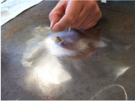
Figure 11: Lift the adhesive tape with the extensor and place the glue on the sheet surface.
