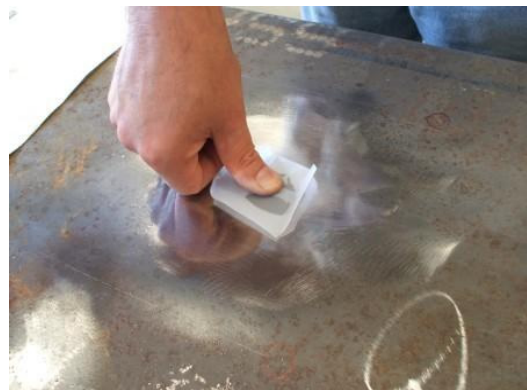
Figure 13: Interpose a little square to avoid direct contact between glue and hands.
