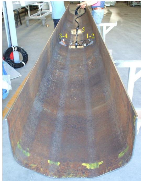
Figure 25: Cure the position of the strain gages so as to be able to detect the deformation state over the entire area.
