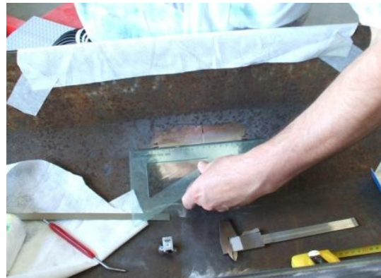
Figure 3: Highlight the geometric lines to help in the correct positioning of the strain gages.
