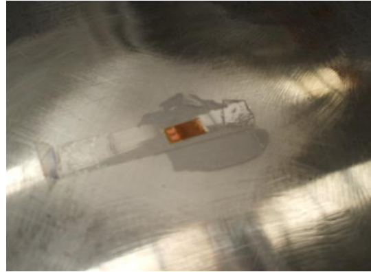
Figure 14: Right: continue to press for the time necessary to solidify the glue and lower the strain gauge.
