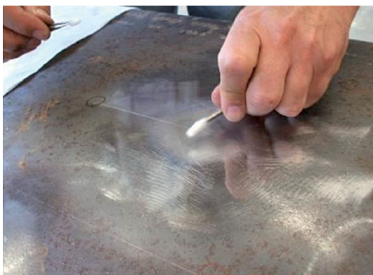
Figure 8: Always cross the passes to get a better cleaning.
