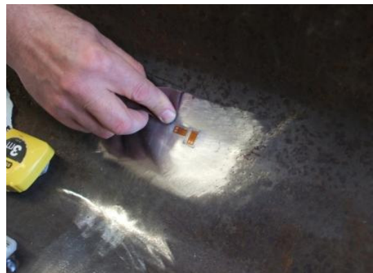
Figure 16: Complete the surface cleaning with sandpaper.
