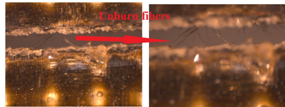
Figure 28. Insufficient burning of fibers in laser cutting
