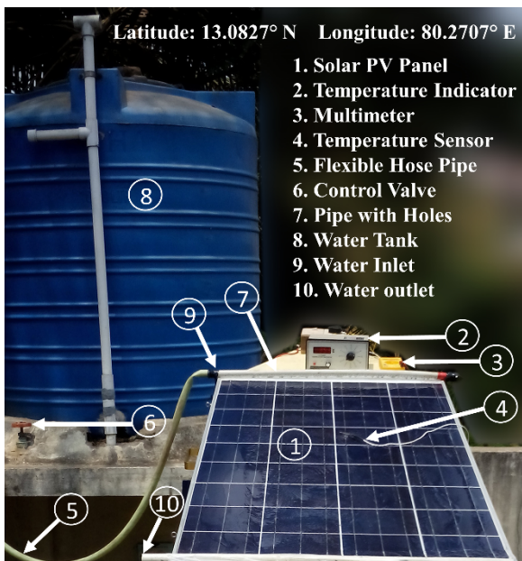
Figure 2. Experimental rig of the PV/T system
