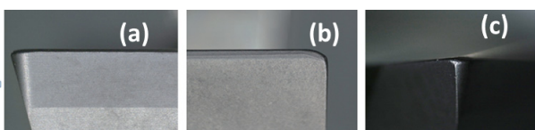
Figure 3: (a) Flank (b) Rake (c) Nose of the insert with K=1.0
