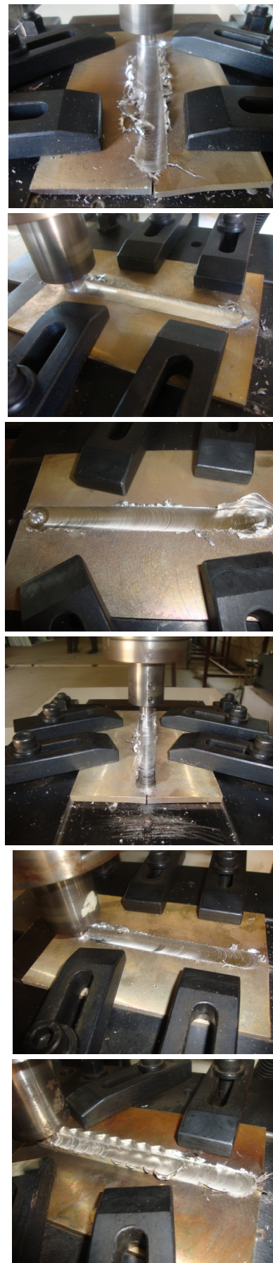
Figure 5. Different flow patterns of the chips arising on the surface of the joints, as the tool shoulder travels over the entire length of the flat plates of AZ80A Mg alloy under different combination of FSW process parameters
