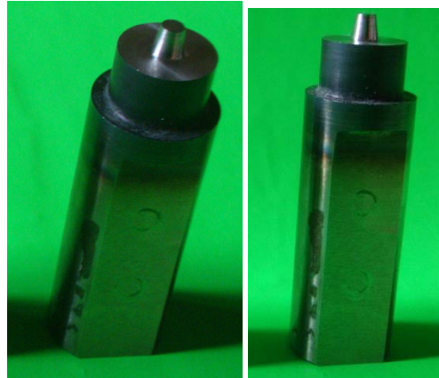
Figure 4. Photographs of the taper cylindrical pin profiled FSW tool employed in this experimental investigation
