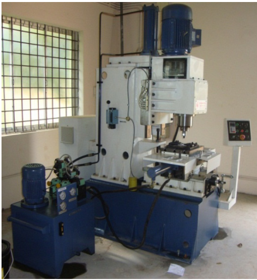
Figure 2. Photographic View of the Friction Stir Welding Machine used in this experimental investigation
