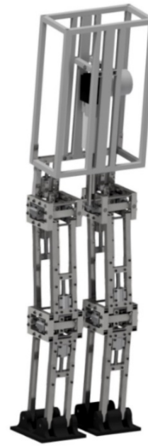
Figure 10. 3D model of the prototype's lower limbs
