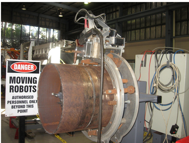
Figure 1. The Girth Welding
