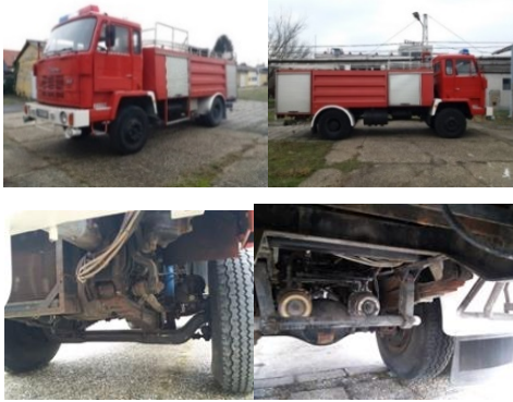
Figure 1. Csepel CSD-755-10 fire truck and its suspension system
