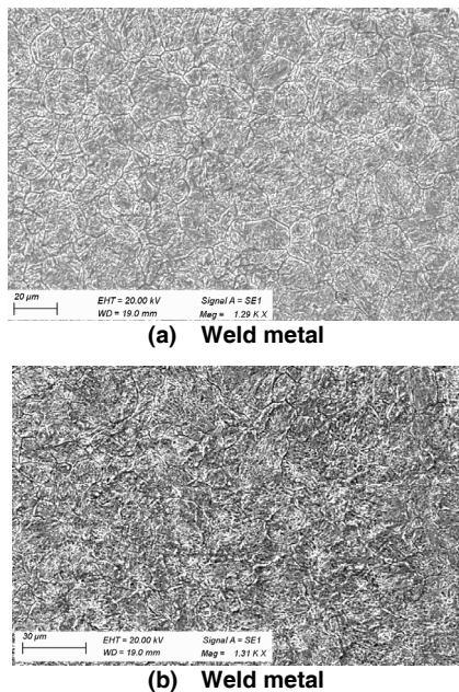
Figure 7 SEM image Argon weld Specimen
