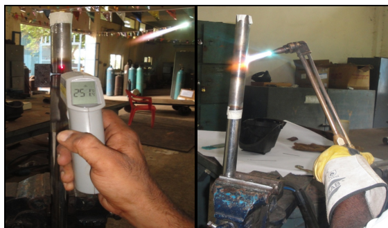
Figure 1: Pre heating the test specimen
