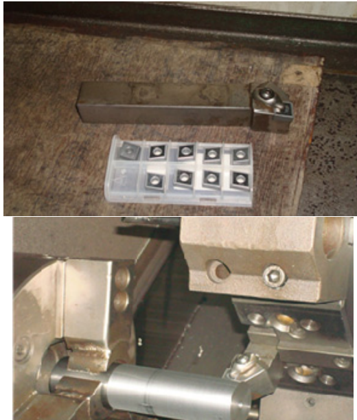
Figure 4. Experimental setup with cutting insert and tool holder
