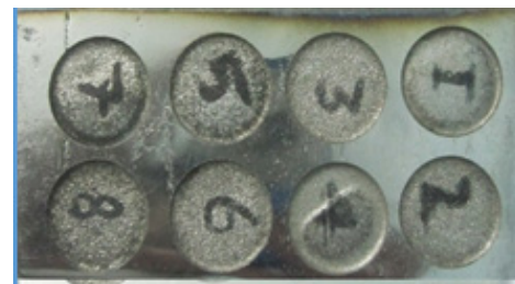
Figure 4. Images of machined Inconel X-750
