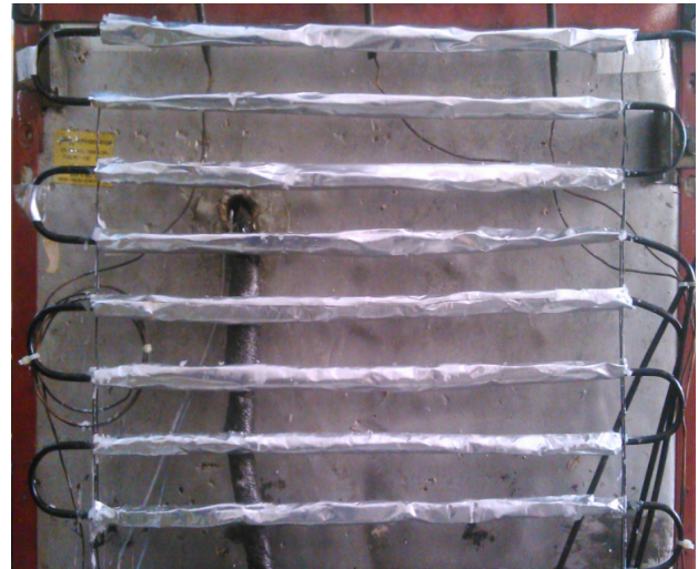
Figure 7. Photographic view of PCM rolled condenser tubes
