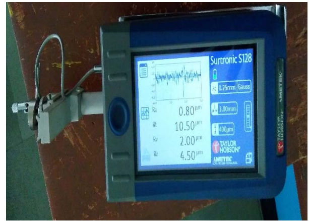
Figure 3. Surface Roughness Tester (Surtronic S128)
