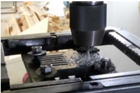
Figure 2. Vertical CNC milling machine setup
