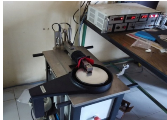
Figure 2. Pin on disc wear test rig
