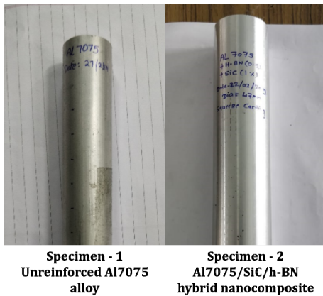
Figure 2. Fabricated squeeze-cast specimens after skinning.
