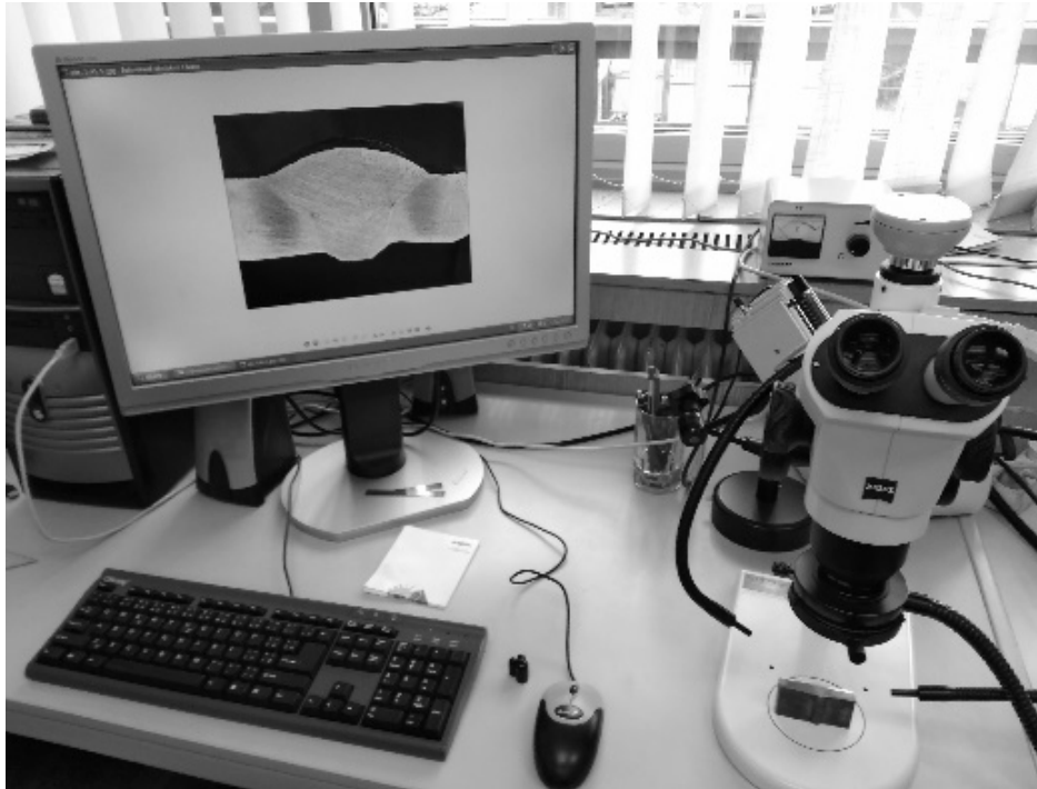
Figure 6. Observation and evaluation of the quality of the weld joints
