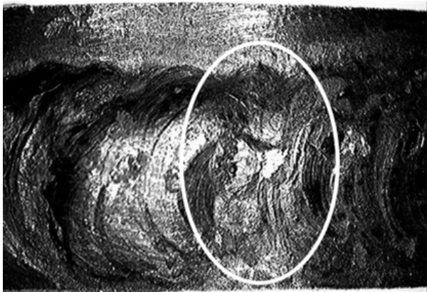
Figure 7. Observation of the defects from the outside of the pipes
