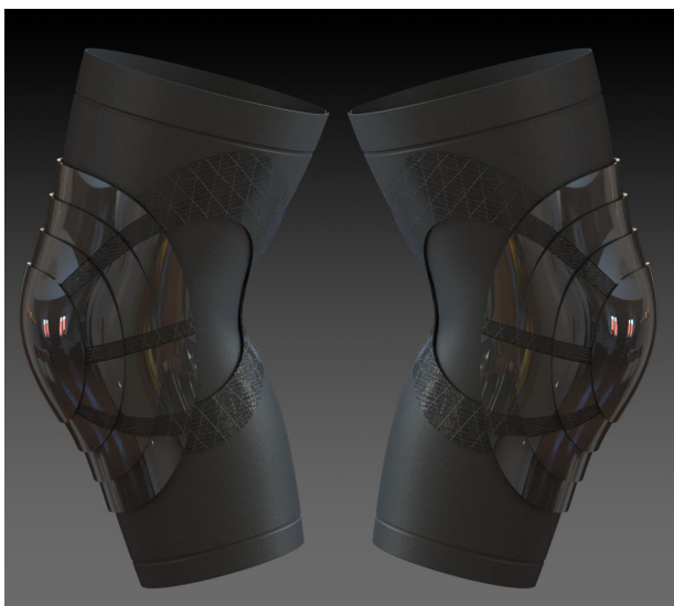
Figure 6. 3D model of the final concept of the knee protector
